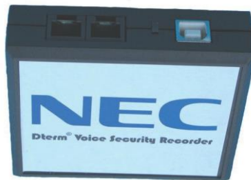
Figure 2-226 1-Port Digital Logging Unit
