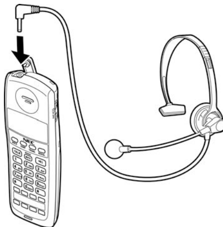
Figure 5-2 Installing the Headset
